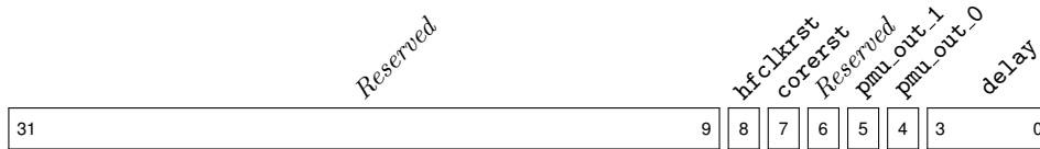
Figure 13.2: PMU instruction format.
